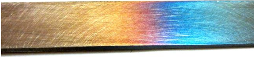
Figure: Differentially tempered steel. The various colors produced indicate the temperature the steel was heated to. Light straw indicates 204 °C (399 °F) and light blue indicates 337 °C (639 °F). [1][2]
