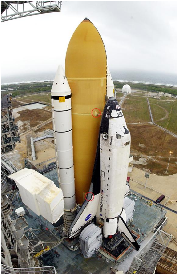
Figure: Columbia prior to launch. The circled area on the external tank (ET) is the left bipod foam ramp, and the circled area on the orbiter is the location that was damaged.
