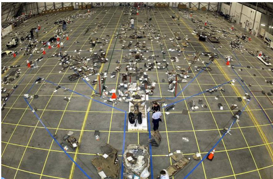
84,000+ parts recovered : A grid on the floor is used to organize recovered debris.
